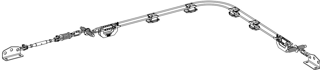
The Travsafe bimaterial version is very similar to the original Travsafe system. It is designed to reduce the higher loading that was generated by the original version. This is done with the use of different kinds of energy absorbers.
